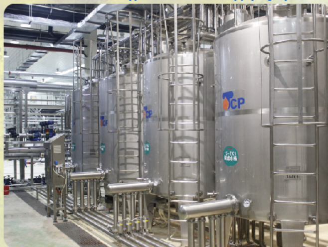
4-Tank Type CIP Solution Supplying System
