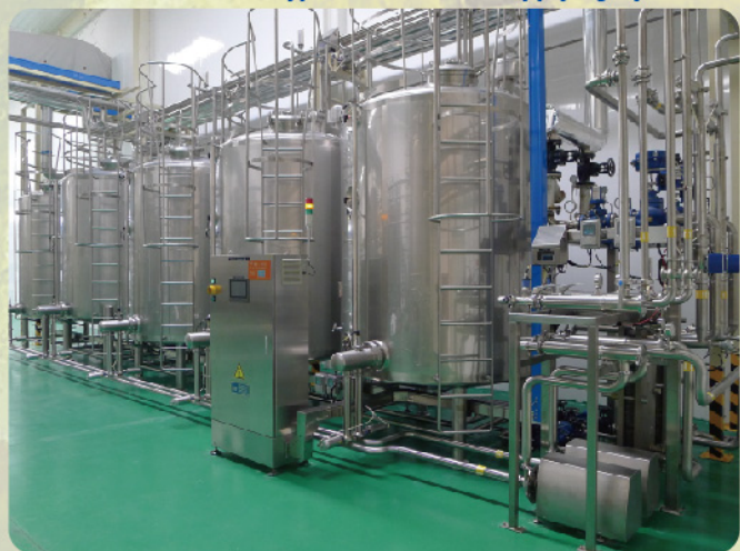
5-Tank Type CIP Solution Supplying System
