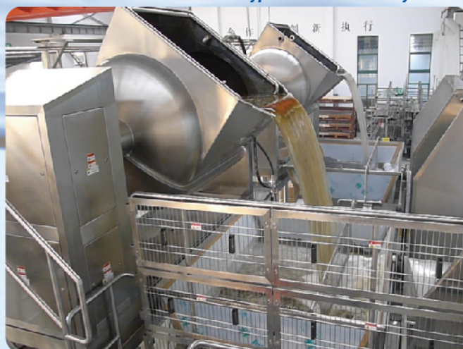
Double Vessel Kneader Type Tea Extraction System
